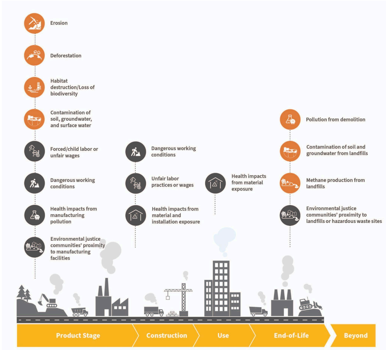
Figure 2-2. Ecological impacts (orange) and human impacts (gray) related to embodied carbon across the life cycle stages of a building. Source: Carbon Leadership Forum (2024) Embodied Carbon 101 .
