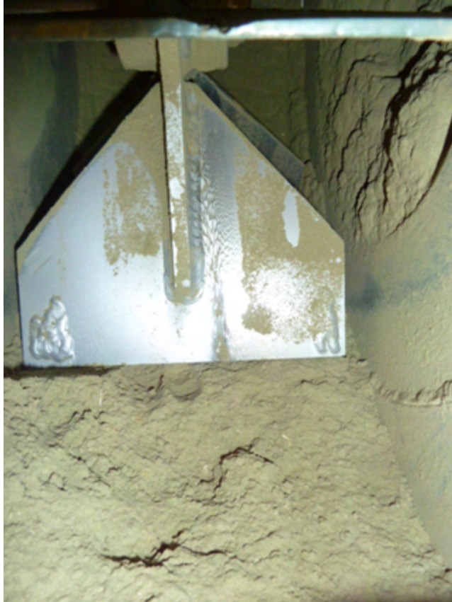
FIGURE C.2. Material settled at the bottom of a fan casing. Image courtesy of The New York Blower Co.
