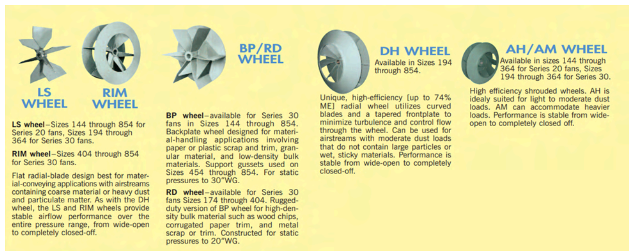
FIGURE C.3. Impeller designs. Courtesy of The New York Blower Co.
