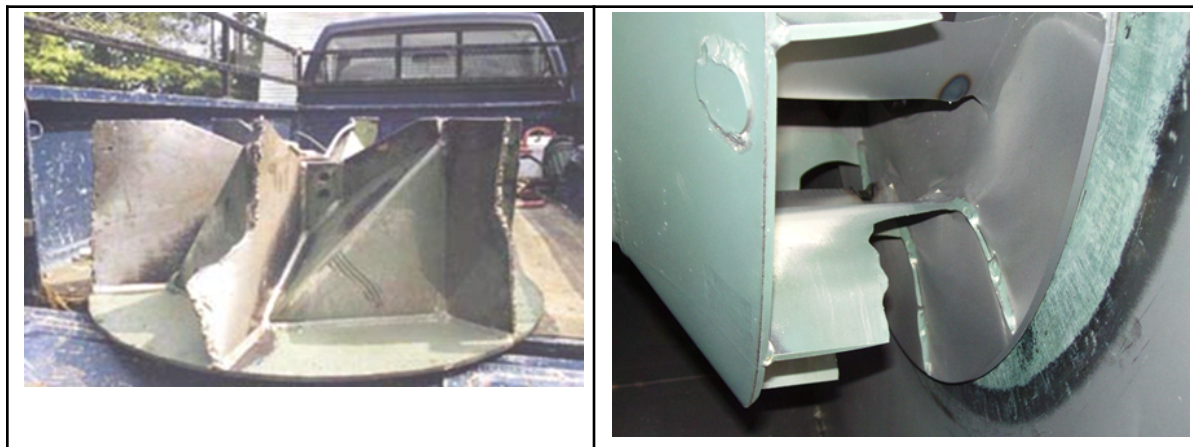
FIGURE C.1. Left: normal wear and tear on an unshrouded radial fan. Right: breakage within a shrouded radial fan installed in an application for which an unshrouded radial fan would have been better-suited.
