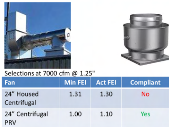
FIGURE 12. How a housed centrifugal fan could be substituted with a rooftop exhaust fan to the detriment of energy savings.
